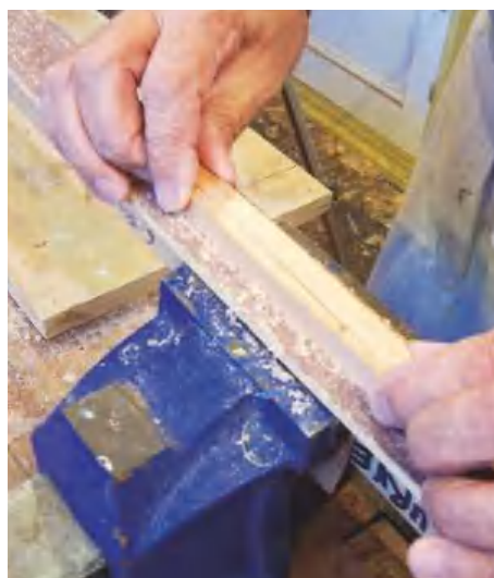
STEP 25. Sanding the curve to give a 3mm lift
